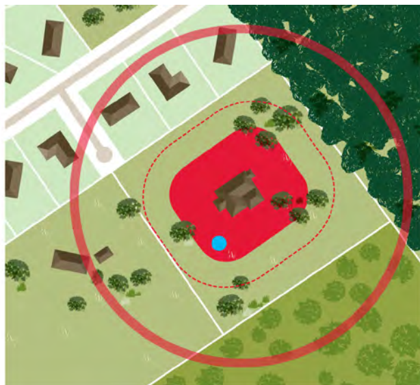
➤ Figure 19: Defendable Space based on worst case aspect for vegetation and slopes. Both inner and outer zone achieved within lot boundaries.
