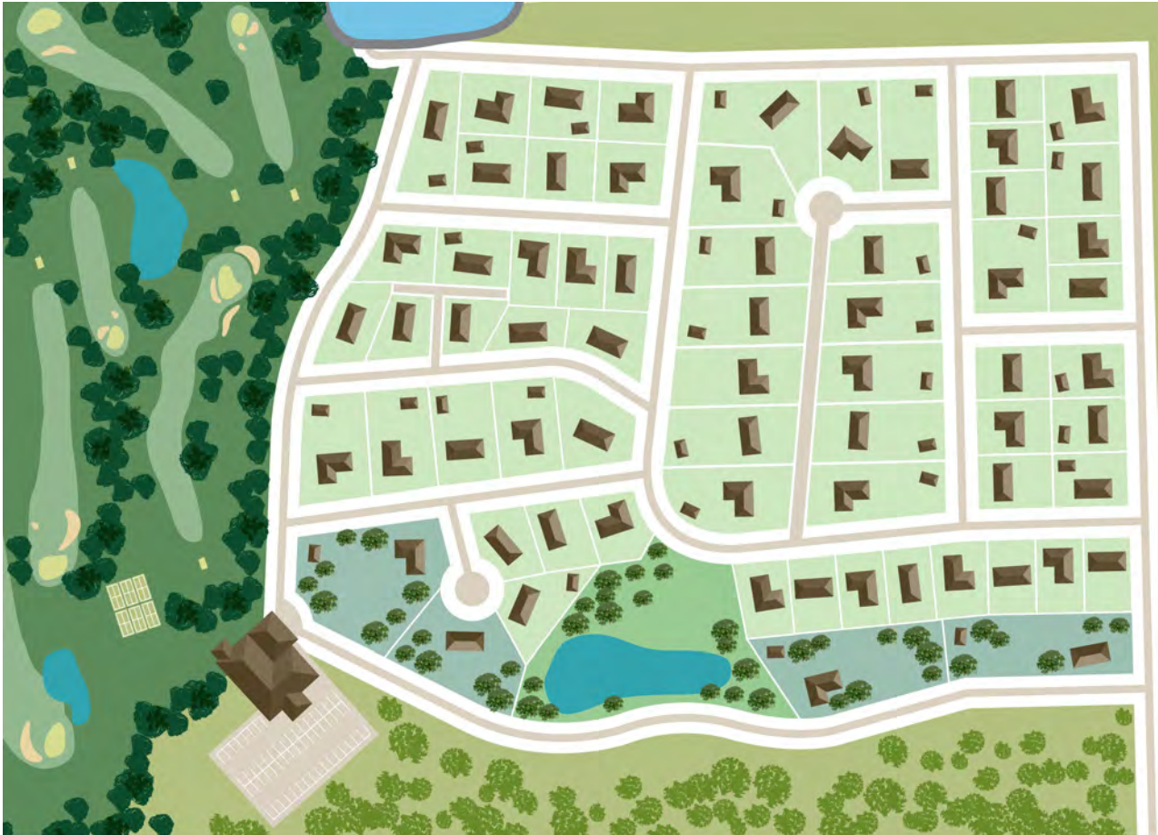
➤ Figure 27: Design components and areas of minimal fuel within a subdivision can be used to help reduce the intensity of a bushfire.
